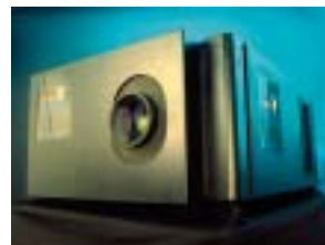
Kodak/JVC projector using D-ILA chips.
